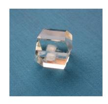
Crystals of  $(NH_4)_2Ln(NO_3)_5$ - $4H_2O$  (Ln = La, Ce) are piezoelectric and pyroelectric and therefore non-centrosymmetric and polar. Crystals with Ln = La, Ce, Pr, Nd are isomorphic and belong to the space group Cc. Large single crystals of the La and the Ce compounds were grown. Their refractive indices and dispersion allow the realization of phase-matching conditions for second harmonic generation.
